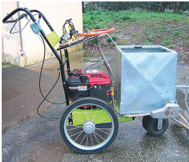
50% with no change in performance. This type of burner turned out to be the best for obtaining a flat, 'brush-shaped' flame guaranteeing high heat transfer and a significant weed-killing effect.
